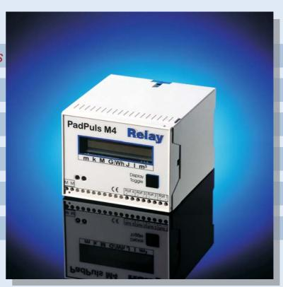
The PadPuls M4 makes up to four conventional meters with pulse output M-Bus compatible in an easy manner. Each of the four inputs can be parameterized practically at will and thus be adapted to existing installations. So the PadPuls M4 combines four M-Bus impulse adaptors in a single unit! It provides the possibility to read actual meter data on-site by the integrated LC display without any auxiliary devices.
