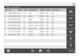
He can start the view of single meters by pushing or clicking on an entry in this list. All options for changing settings are locked. The only action he can do is reading the current data of the meter by clicking on the button "Read Values" in the "Values" tab.
