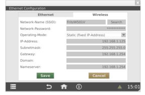
The "Wireless" configuration is similar to the "Ethernet" (RJ45) configuration. There is an additional search for WIFI networks followed by a selection of the WIFI access point (AP) and an input field for the password.
