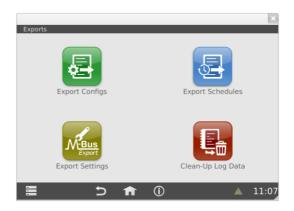
M-Bus Export The button "M-Bus Export Settings" opens a dialog where you can select in the sheet "format" the decimal delimiter for numbers, which can be either a "comma" or a "point / dot". You can also limit the size of the database to a specified number of days. The device then automatically
