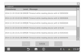
The entries in the log book can show for example errors occurred during communication in M-Bus. The above example shows a meter which could not be read several times during logging. A short circuit on the M-Bus is also a possible error message. Another example of possible error messages is that the device could notify a failed synchronisation of the clock from a time server in the internet.
