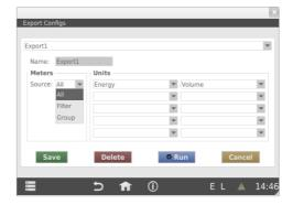
The most important values energy and volume are selected in the above example. There are further possibilities to choose the data of all meters (All) or meters from a predefined filter (Filter, e.g. all electricity meters) or meters from a specific group or tenant. The created export config can be saved under a name for further use with "Save". The button "Run" starts the export immediately:
