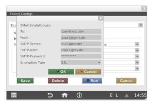
You have to enter the destination e-mail address and the SMTP server in case of an e-mail transfer. If you want to use your internal Microsoft exchange server, please enter the IP address of that server and the exchange user with password. The encryption type for MS Exchange is "Plain" (unencrypted). The example shows the settings for a GMX account using the GMX SMTP server. The e-mail sending with GMX needs encryption (Encryption Type = "SSL").
