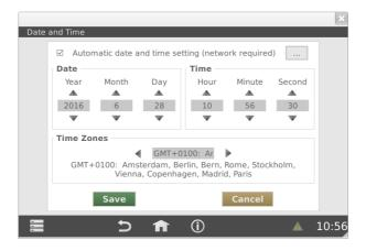
If the option "automatic date and time setting (network required)" is activated, the WebLog synchronizes the internal clock once per day with the clock of a time server in the Internet. By a click on the button with the
