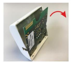
To connect the cable, first tilt the circuit board out of the top shell by pulling on top of the edge of the semicircular notch on the circuit board.
