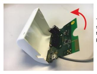
The cable is then led back through the lower semicircular notch of the circuit board. Then insert the PCB at the bottom and tilt it up until it clicks into place.
