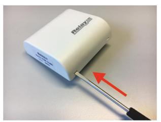
The housing must first be opened for assembly. To do this, push the tip of a slotted screwdriver one after the other into the two openings on the lower side so that the locking mechanism of the cover is released from the mounting plate.
