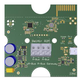
Now connect the M-Bus cable to one of the two removable terminals. The printed circuit board with the terminals can be seen in the picture opposite.
