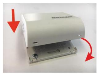
Finally, the housing cover incl. printed circuit board is clipped onto the already mounted mounting plate. To do this, attach the lid to the top edge of the mounting plate and press the lid firmly onto the plate until it snaps into place.
