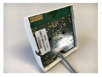
The housing cover with the latched circuit board and connected cable looks like this:
