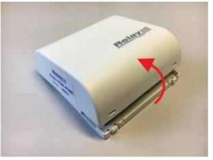
Subsequently, the upper shell can be lifted off the mounting plate.
